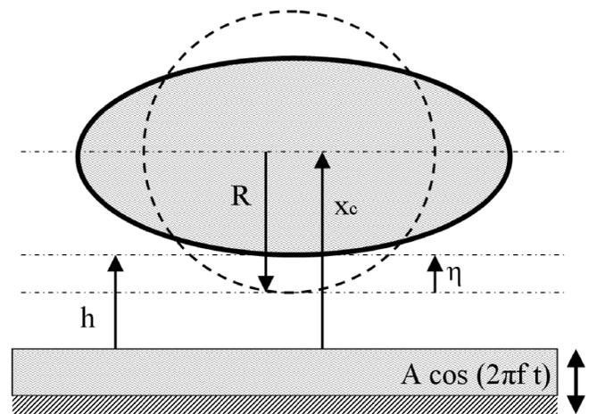
FIG. 2. Geometrical variables needed to model a bouncing droplet of undeformed radius  $R$ :  $x_c$  is the distance between the droplet center of mass and the bath,  $h$  is the minimum air film thickness, and  $\eta$  is the vertical droplet deformation about the axis of symmetry.
