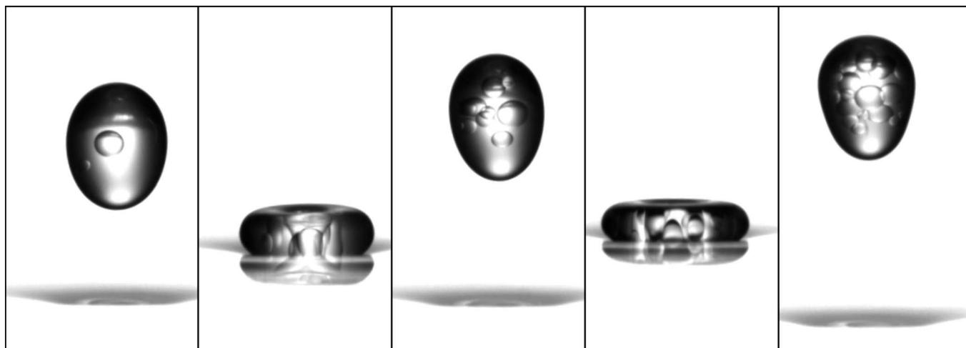
FIG. 2. Bounce after bounce, small oil droplets are created within the water droplet, thus progressively forming a microemulsion of oil-in-water-in-oil.
