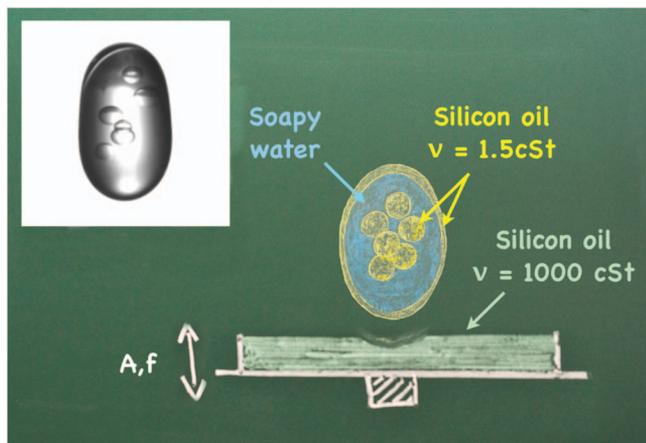
FIG. 1. (Color) Experimental setup. A millimetric compound droplet bounces on a high viscosity oil bath which is vibrated vertically (sinusoid of amplitude  $A$  and frequency  $f$ ). When the amplitude is sufficiently high, the oil layer penetrates into the water droplet, thus forming a double emulsion (enhanced online). [URL: <http://dx.doi.org/10.1063/1.3202626.1>]
