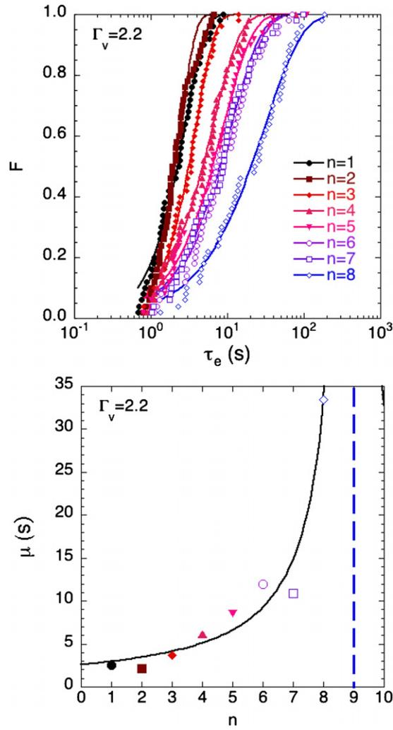
**Figure 4.** Top: cumulative distribution function  $F$  of escape times  $\tau_e$  of one bead out of a compartment containing  $n$  beads when  $\Gamma_v = 2.2$  (see the legend). Bottom: mean value of  $\tau_e$  from equation (4) as a function of the number of beads contained in a compartment. The curve is a fit using equation (5). Note that the symbols used for the top and bottom figures are the same.
