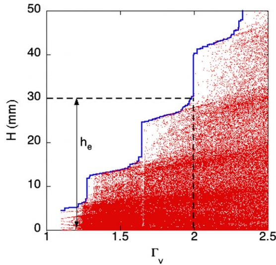
**Figure 3.** Heights reached by a bouncing ball with a coefficient of restitution equal to 0.83 with respect to the acceleration  $\Gamma_v$  at 25 Hz. The horizontal line represents the height of a compartment at 30 mm and the height for which the centre of mass of the bead may be higher than the height of a compartment. The continuous line represents the envelope curve and consequently the maximum reachable height for the bead at the considered acceleration.
