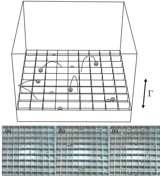
**Figure 1.** Top: schematic view of the 9 by 9 grid. Bottom: snapshots of the grid during a sweep in acceleration (at 25 Hz) between  $\Gamma_v = 0$  to 4. (a) Initial state, one bead per compartment, (b) clustering state and (c) gas state when  $\Gamma_v = 4$ . A movie can be seen at the link [3].
