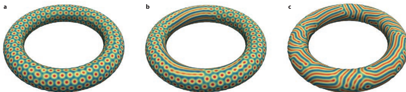
Fig. S2: Wrinkling morphologies on a toroidal geometry with R_1 = 80 and R_2 = 16 for increasing excess film stress: (a) \Sigma_e = 0.25 , (b) \Sigma_e = 0.5 and (c) \Sigma_e = 2.0 . As in spherical geometries, one observes a transition from hexagonal to labyrinth-like patterns with increasing excess stress \Sigma_e . However, in contrast to the spherical case, the non-constant curvature on the torus can lead to local symmetry-breaking, i.e., at intermediate values of \Sigma_e labyrinth patterns are more likely to emerge at the inner saddle-like regions of the torus, see (b), whereas hexagons remain stable in the outer regions of the torus, where the two principal curvatures have the same sign resulting in a larger mean curvature. Simulation parameters are \gamma_0 = -0.079 , c = 0.075 , (a) a = 0.017 , (b) a = 0.016 , and (c) a = 0.007 , using an unstructured surface triangulation with > 26,000 nodes.
